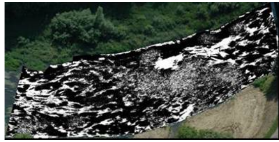
Fig. 42 : Result of Image analysis on figure 41
