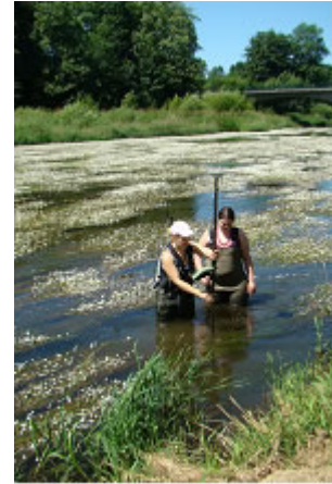
Fig. 38 : DGPS systems on the field: measurements in the Semois river with the rover
